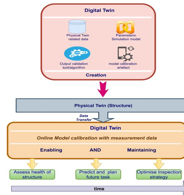
Fig 5: DT creating, enabling and maintaining process with model validation and adaptation/calibration artefact.
