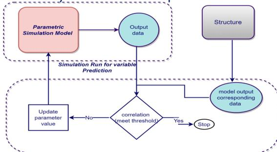
Fig 2: model calibration with parameter updating with model output and structural data comparison.
